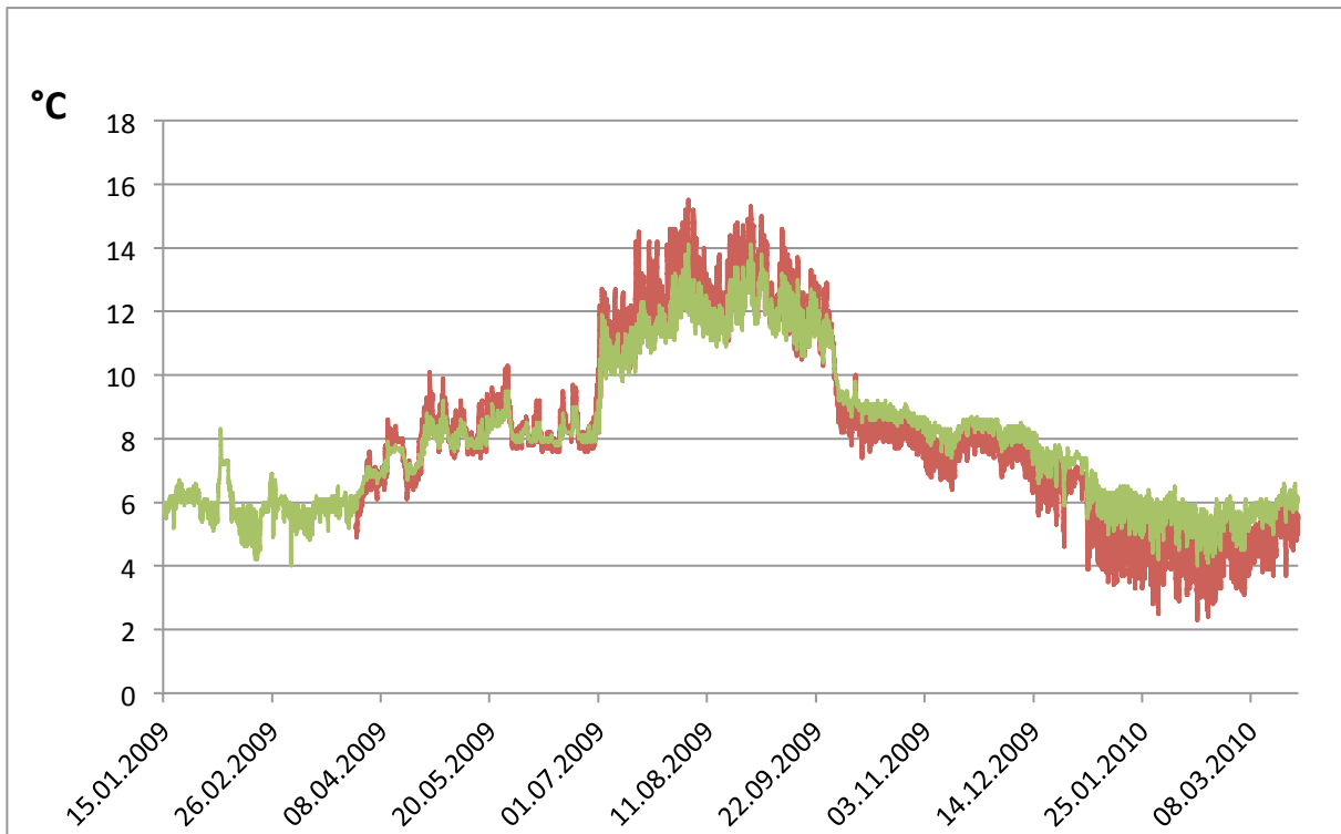
Figure 9 Borehole temperatures in BH 4 at 50 m (green) and 100 m depth at the IKEA BTES plant in Uppsala.
