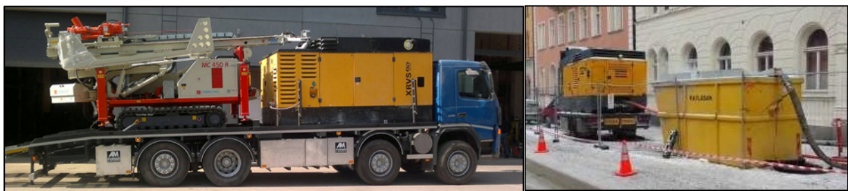
Figure 4. Left, a normally sized drilling rig and a 30 bar compressor. Right, set up for drilling showing the compressor and container for separation of cuttings. The hose hanging down from the container is connected to the rig out-blow.
