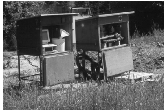
Figure 5: The German (Landtechnik Weihenstephan) thermal response test rig. Photo: Landtechnik Weihenstephan
