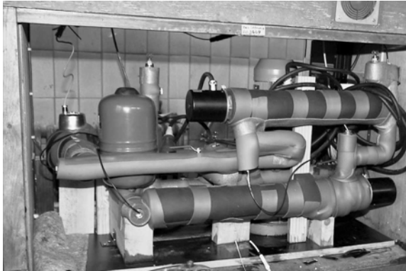
Figure 5: The German (Landtechnik Weihenstephan) thermal response test rig. Photo: Landtechnik Weihenstephan
