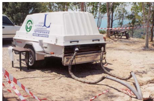
Figure 8: The Turkish response test rig was built in Sweden and is of the TED-model. Photo: Bekir Turgut.
