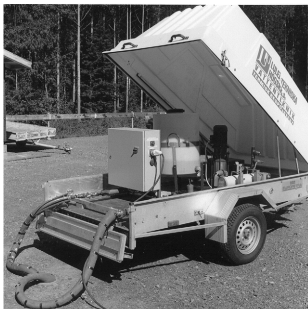
Figure 2: The Swedish response test rig (TED). Photo: Peter Olsson.
