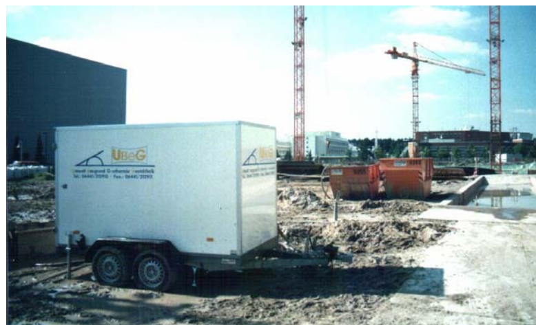
Figure 4: The German (UbeG) thermal response test rig. Photo: UBeG GbR, Wetzlar
