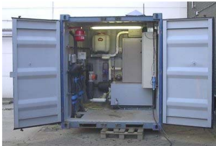
Figure 6: The Dutch response test unit with cooling and heating mode. Photo: Groenholland.
