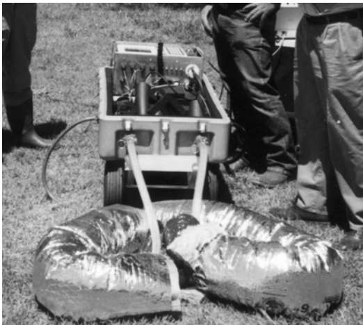
Figure 11: The suit-case response test set-up of Ewbanks, USA. Photo: Signhild Gehlin.
