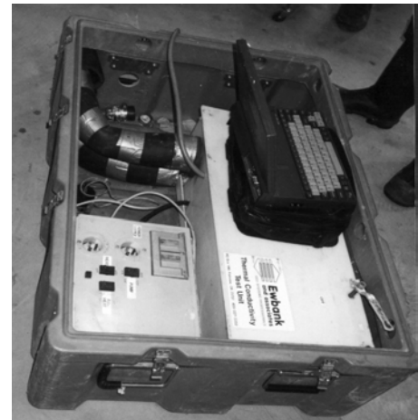
Figure 11: The suit-case response test set-up of Ewbanks, USA. Photo: Signhild Gehlin.
