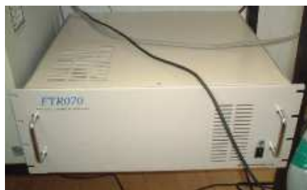
Figure 2.2: Optical fiber temperature laser radar.
