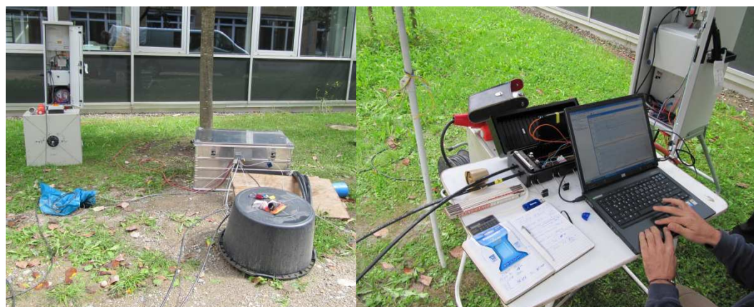
Figure 3.4: ERGT with measure device and data logger.
