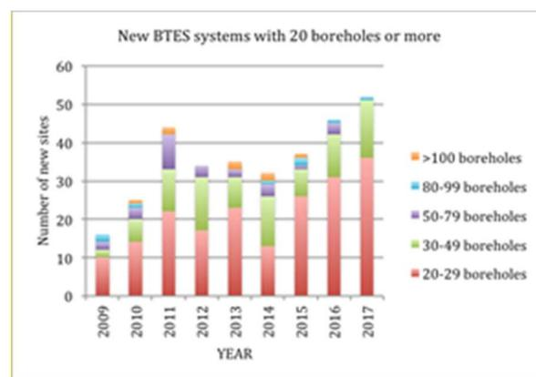
**Figure 6: New large plants dominated by BTES 2009-2018 registered in the SGU Well Database (SGU Well database 2019).**
