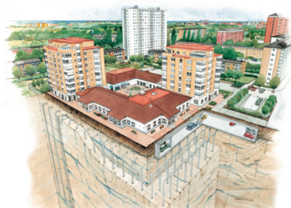
Figure 5: Borehole Thermal Energy Storage (BTES). Illustration: Geotec.
