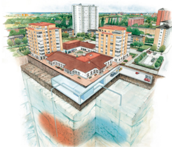
Figure 4: Aquifer Thermal Energy Storage (ATES). Illustration: Geotec.
